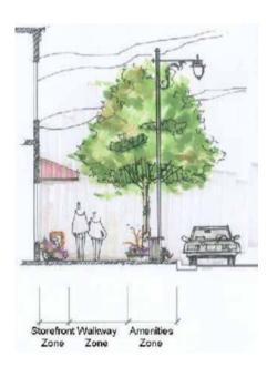
Walkway zone. The 4-foot wide walkway zone is the middle section of the sidewalk. Its primary function is to accommodate the efficient movement of pedestrians. As such, it needs to provide an unobstructed, linear sidewalk space that is free of any street furniture or public amenities.
